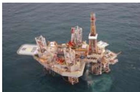
**ENSCO 60 before its reconvention in JAHWRA 5, Jack-Up, Mobile Offshore Drilling Production Unit**
