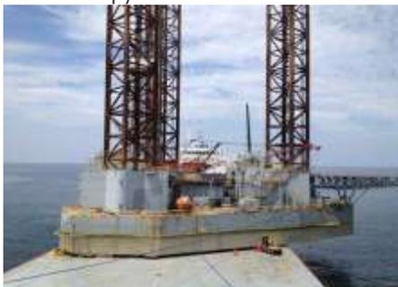
*The Jack up Rig and the Jacket, on the semi-submersible*
