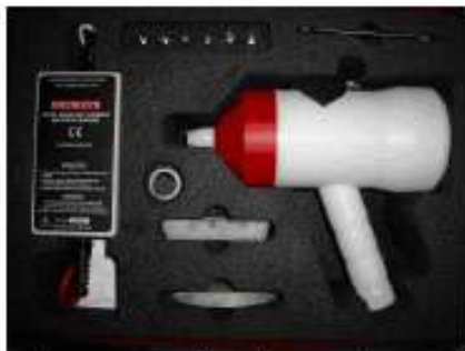
Roxby apparatus for underwater Cathodic Protection measurements
